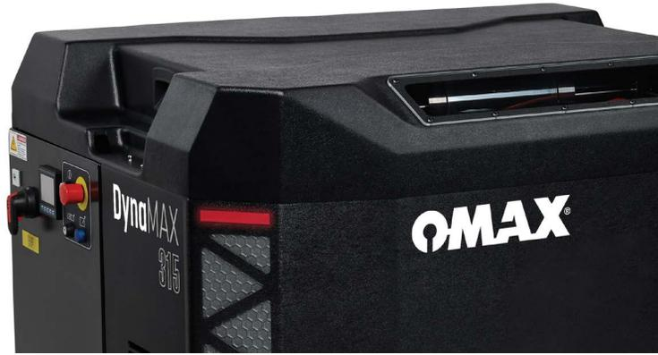
DynaMAX 3-series pumps include the next evolution of Advanced Intensifier Technology (AIT) that eliminates soft, static high-pressure seals and incorporates industry-leading cartridge seal design, **enabling rapid replacement of common consumables**. A closed-loop proportional pressure control adjusts for ambient pressure and temperature, oil viscosity and hydraulic system wear parts, to **deliver consistent quality at optimum cutting speeds**, all in a reduced footprint design.
